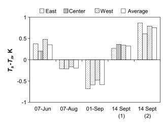
**Figure 4** Temperature differences between the southern (inlet) and northern (outlet) sides of the reservoir. Bar patterns represent different thirds of the reservoir, and blank bars represent the average. Each data set (cluster of four bars) was calculated based on profiles measured at 9 cells. Hours of data collection: June 7 - 13:00; August 7 - 09:00; September 1 - 09:00; September 14(1) - 08:30; September 14(2) - 12:00.
