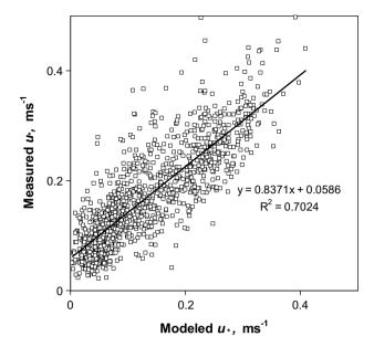
**Figure 1** Friction velocity calculated directly from the measurements (Eq. (4.5)) plotted against that predicted by the logarithmic wind profile model (Eq. (4.2)). The solid line is the least square regression line, where y = 0.84x + 0.06 ( $R^2 = 0.7$ , 1176 data points).
