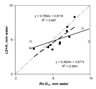
**Figure 5** Dissipated versus available energy. The light dashed line has a 1:1 slope. The solid line was fitted to all data points using the least squares technique with the equation y = 0.36x + 3.67,  $R^2 = 0.39$ . The heavy dashed line was fitted to the full square data points only with the equation y = 0.8x + 0.8,  $R^2 = 0.69$ . The empty squares represent days with significant deviation from the 1:1 line.
