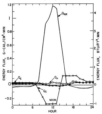
Fig. 5. The daily pattern in net thermal radiation  $(Q_{NR})$ , evaporation  $(Q_R)$ , convection  $(Q_R)$ , and conduction  $(Q_G)$  for the nonforested H. J. Andrews study section.
