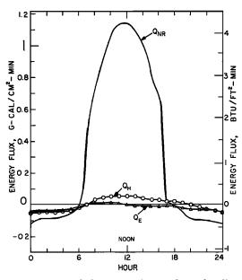
Fig. 3. The daily pattern in net thermal radiation  $(Q_{BB})$ , evaporation  $(Q_B)$ , and convection  $(Q_H)$ for the nonforested Berry Creek study section.
